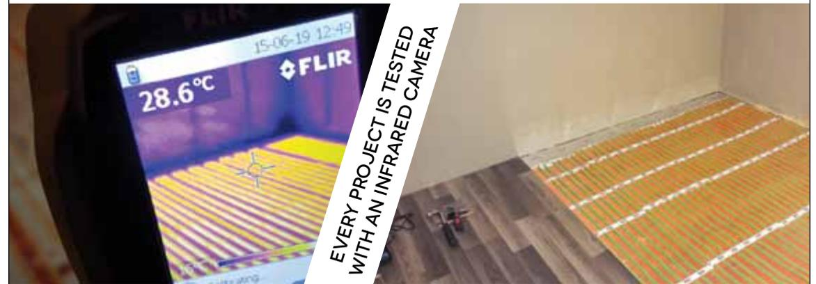
EVERY PROJECT IS TESTED WITH AN INFRARED CAMERA
