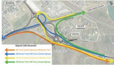
its. East/west and north/south regional traffic flow will continue to operate as it does today and drivers will not be impeded by local traffic. The Sarcee Trail bridge deck over the TCH will be rehabilitated and reconfigured for better safety and efficiency; the west bound ramp on and off of the TCH will also be upgraded. Please reference the diagram.
